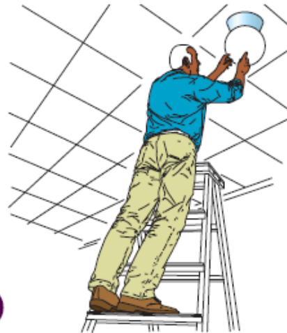
Figure 4a Correct - three clear steps. Don't work any higher up this type of stepladder
