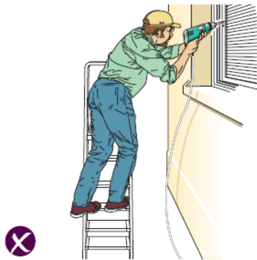
Figure 3b Incorrect - rungs side-on to work activity
